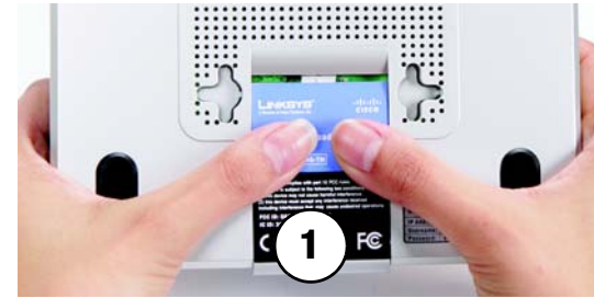
Figure 4-11: Slide Down the SIM Card Cover
